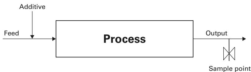
Figure 5.1 Chemical injection and sampling process
